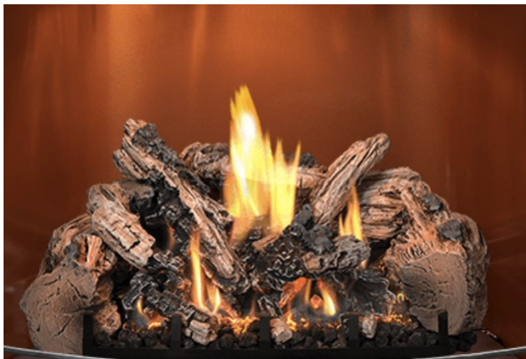
Figure 6-2 Burner Flame Heights: This image provides a visual reference for the burner flames burning at maximum height after the burners have been operating for 30 minutes or longer. A normal rear flame will be 1 to 2 inches above the rear log top edge. This, however, is dependent on the gas type, air shutter opening setting and vent system configuration. Actual flame heights can be slightly higher or lower when compared to this reference image.
